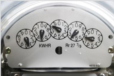
When reading an electric meter, read and write down the numbers as shown on the dials from *right to left*. When the pointer is directly on a number, look at the dial to the right. If it has passed zero, use the next higher number. If the dial has not passed zero, use the lower number.
